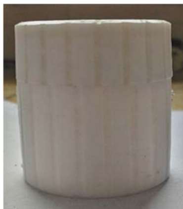
Figure 2. Volatilization chamber made of teflon
