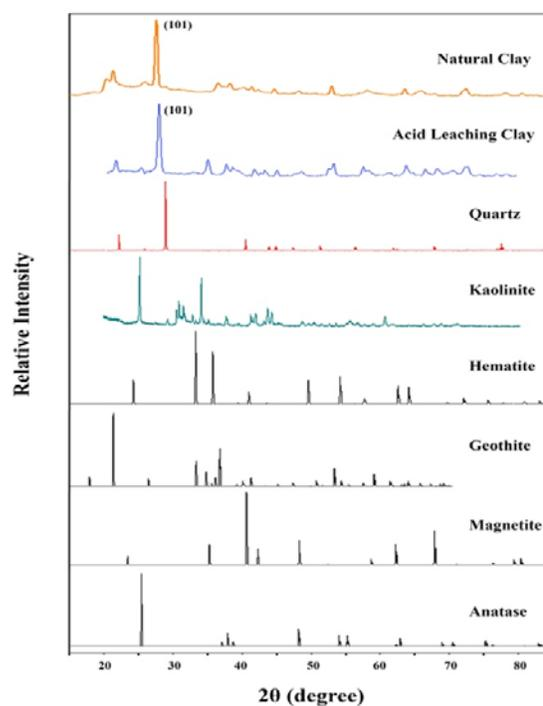
Figure 1. Diffractogram natural clay and acid leaching clay
