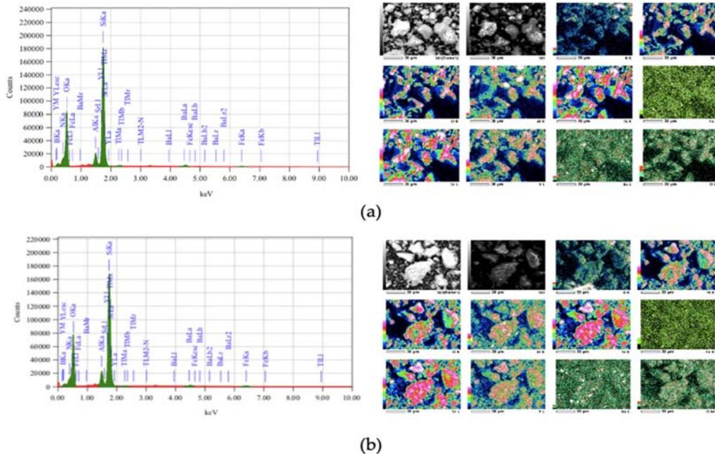
Figure 3. EDS mapping analysis of (a) natural clay and (b) acid leaching natural clay
