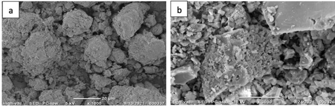
Figure 2. Samples morphology using SEM 5 kV with magnification 1000× (a) natural clay (b) acid leaching clay
