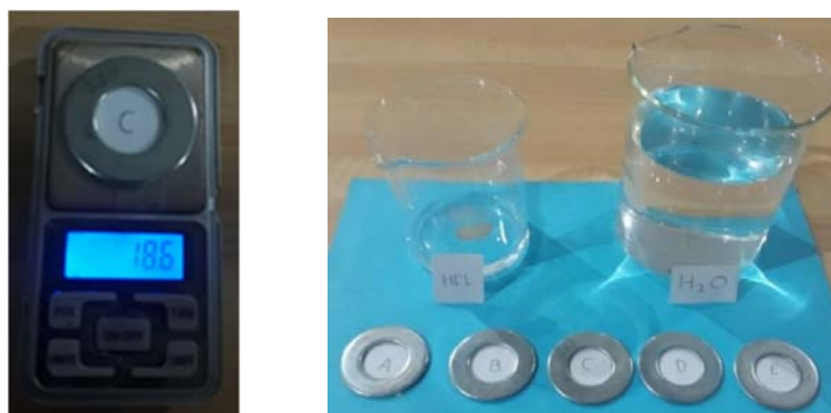
Figure 2. Test for zinc-coated thickness using hydrochloric acid solutions
